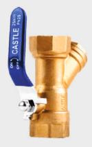
Castle Ball Valve with Strainers is used in HVAC and Plumbing sectors. These valves are extensions of Castle Ball Valves. The strainer performs the function of removing the particulates from the fluids passing through it via the filtering element intersecting the main channel. The strainer consists of a cylindrical mesh that protects the valuable downstream equipment's such as pumps, regulators etc. from being damaged from the contaminants.
